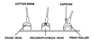
When the heads, capstan and pinch roller become dirty, this may result in muffled, distorted or reduced sound during playback and may even result in tape jams.
